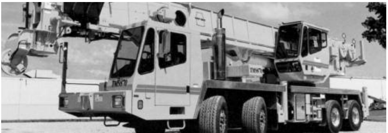
Mobile crane using a Sprag Clutch on the boom raise and lower mechanism, holding the weight of the boom against the diesel engine drive in the lowering motion preventing overspeeding.
